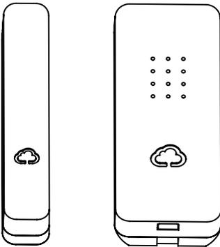
**Step 2.** Rotate the magnet so that the logo are aligned in the same orientation, place it on the **left** side of the main sensor element.
