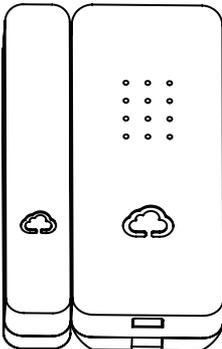
**Step 3.** Move the magnet in contact with the Reed KumoSensor and then away. A LED light should start flashing for about 2 minutes. Search and associate during that time.
